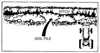
Operate at right angles to the ditch. Take as big a bite as the tractor can handle without lugging down.
